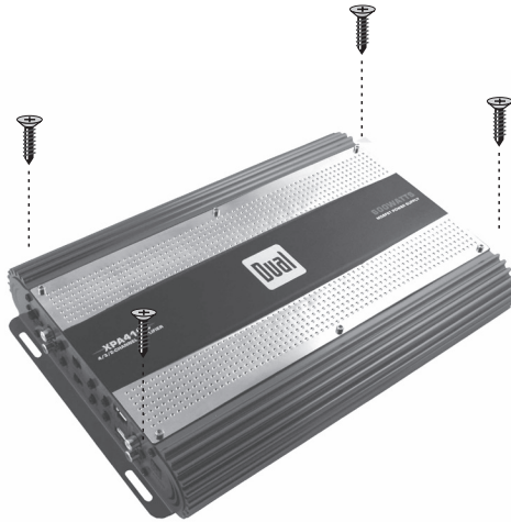
TYPICAL MOUNTING METHOD
